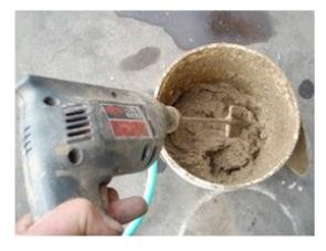
If you have access to electricity, a drill with a paint mixer attachment is a quick, satisfactory way to remove lumps in wet clay. Depending on the condition of the clay you may need to soak it several days.
