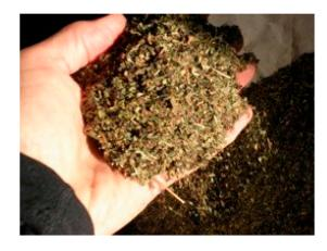
Rice hulls, sawdust, pumice, screened fresh stable manure and a variety of other materials also work to mix with clay to create an insulated and durable mud Rocket Stove.
