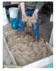
The better the ingredients are mixed together, the more durable the stove will be and the longer it will last. Incomplete mixing will result in a stove that will crumble.
